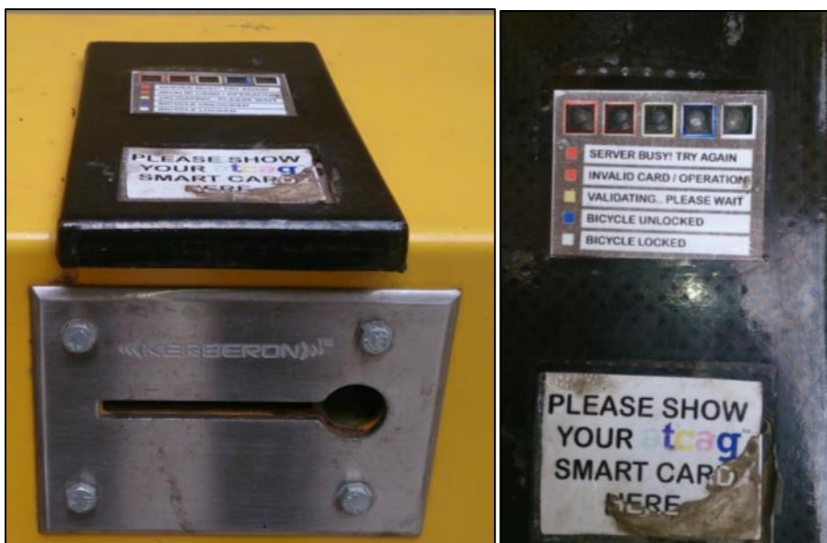
Figure 9 Locking/Unlocking Mechanism of ATCAG docking station
