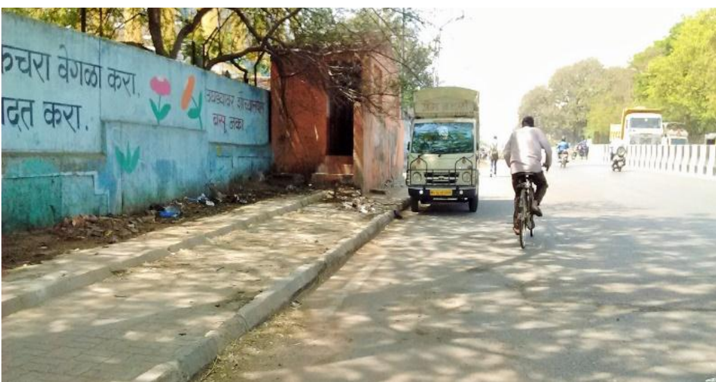
Figure 9: Cyclists being forced to use the carriage way because of unplanned services in the NMT lanes (like public toilets)
